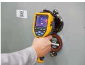
Combine with a Fluke ClirVu™ Infrared Window to conduct thermal inspections without having to open the electrical panel.
